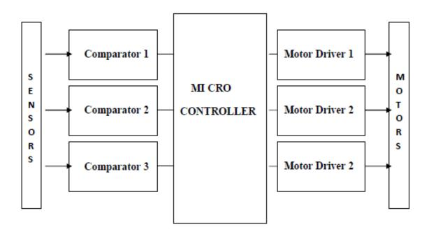
At initial position all the wheels are on the ground and microcontroller is programmed in such a way that the robot moves forward till the sensor circuit detect any obstruction. The sensor circuit consist of IR LED and phototransistor. The IR LED emits the IR radiations ,when there no obstruction the phototransistor does not detect any reflected radiation and the vehicle moves forward without any vertical motion.
